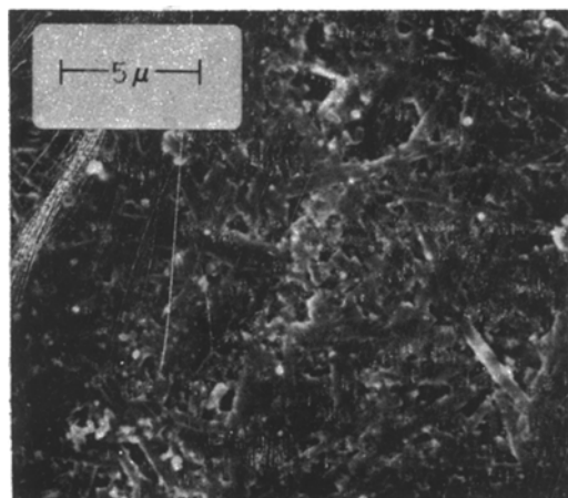
Fig. 2. SEM-photo of a pressed and sintered \text{TiO}_2(\text{B}) -electrode.
